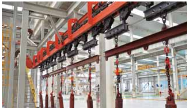
An automatic painting production line of oil pressure levers in a smart factory 智能工廠裏的立柱、千斤頂自動塗裝生產綫
