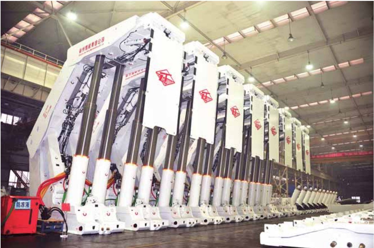
8.8m Hydraulic Roof Support, independently developed and manufactured by ZMJ 鄭煤機自主研發製造的8.8m液壓支架
