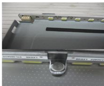
侧光式LED背光源 (Edge LED)
