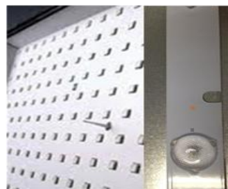
直下式LED背光源 (Direct LED)
