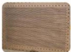
舰船换热器用铜复合板 Copper and steel composite plate for naval heat exchanger
