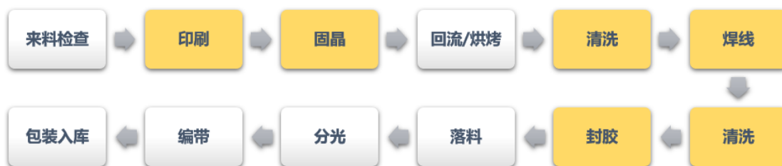
(3) 灯丝及 COB 封装器件工艺流程图
