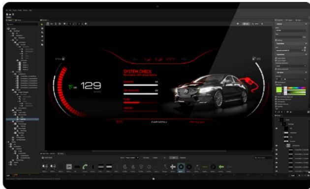
Figure 15: An in-vehicle digital instrument cluster designed by using Kanzi Studio
