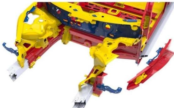
Figure 5 (Front components, exploded view of Shotgun)
