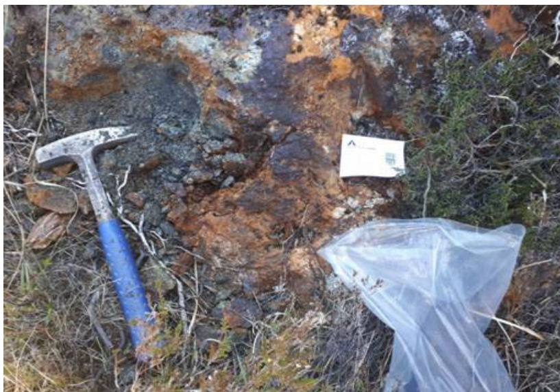
Figure 4: Second outcrop at Kerry Road deposit with visible chalcopyrite, 30 metres northwest of main outcrop, grading 2.16 g/t Au, 14 g/t Ag, 5.23% Cu and 0.30% Zn. Photo and data obtained from GreenOre.
