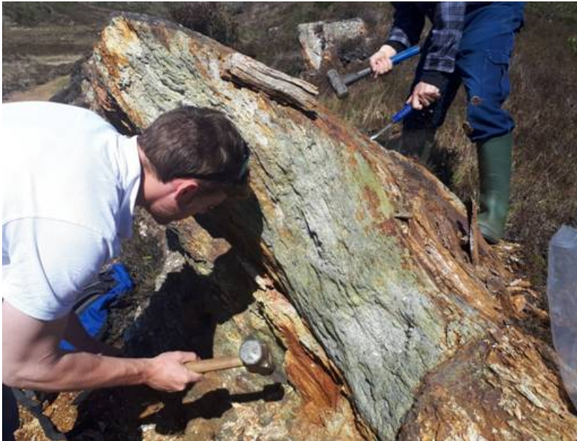
Figure 4: Second outcrop at Kerry Road deposit with visible chalcopyrite, 30 metres northwest of main outcrop, grading 2.16 g/t Au, 14 g/t Ag, 5.23% Cu and 0.30% Zn. Photo and data obtained from GreenOre.
