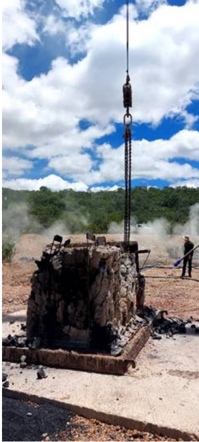
Stacked coking ovens 'cooking' the coal at 900-1,100°C
