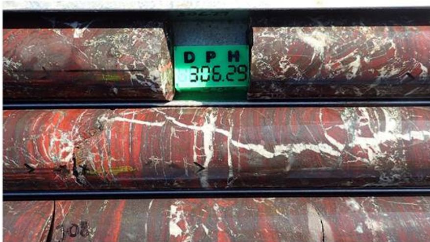
Figure 1 - Example of highly altered & structurally deformed Banded Iron Formation at 306m depth in Hole DITDD004, indicative of a possible Lode Gold System
