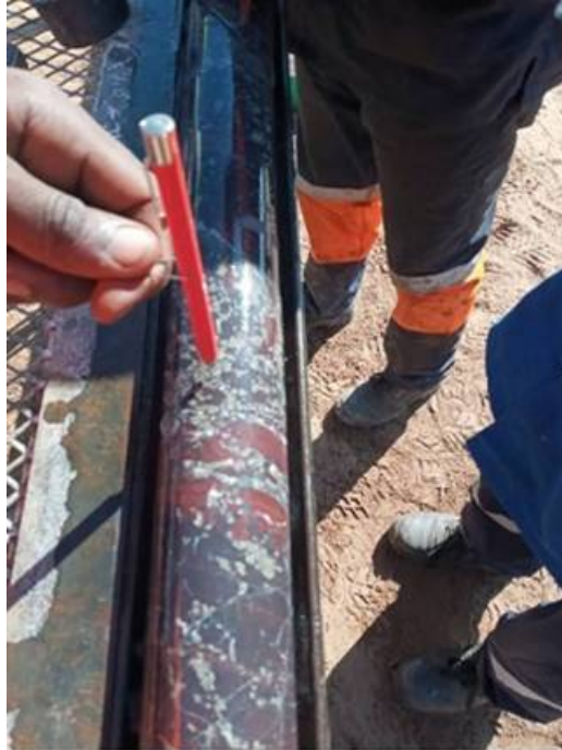
Figure 2 - Strong response from magnetic pencil used over the 100m thick BIF encountered in DITDD004.
