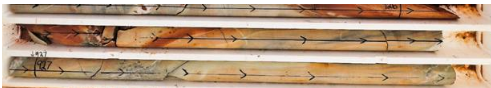
Figure 4: RAD002 - Angular unconformity, breccia - quartz vein contact at 924m; into the mineralised and oxidised calc-arenite sedimentary sequence
