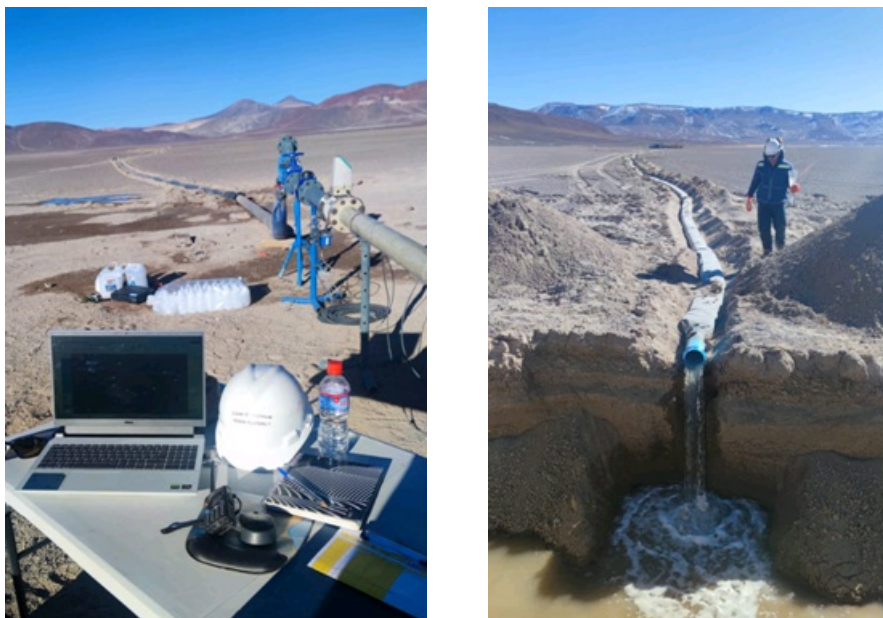
Figure 2: Pictures of FB01 Pump Test in Progress
