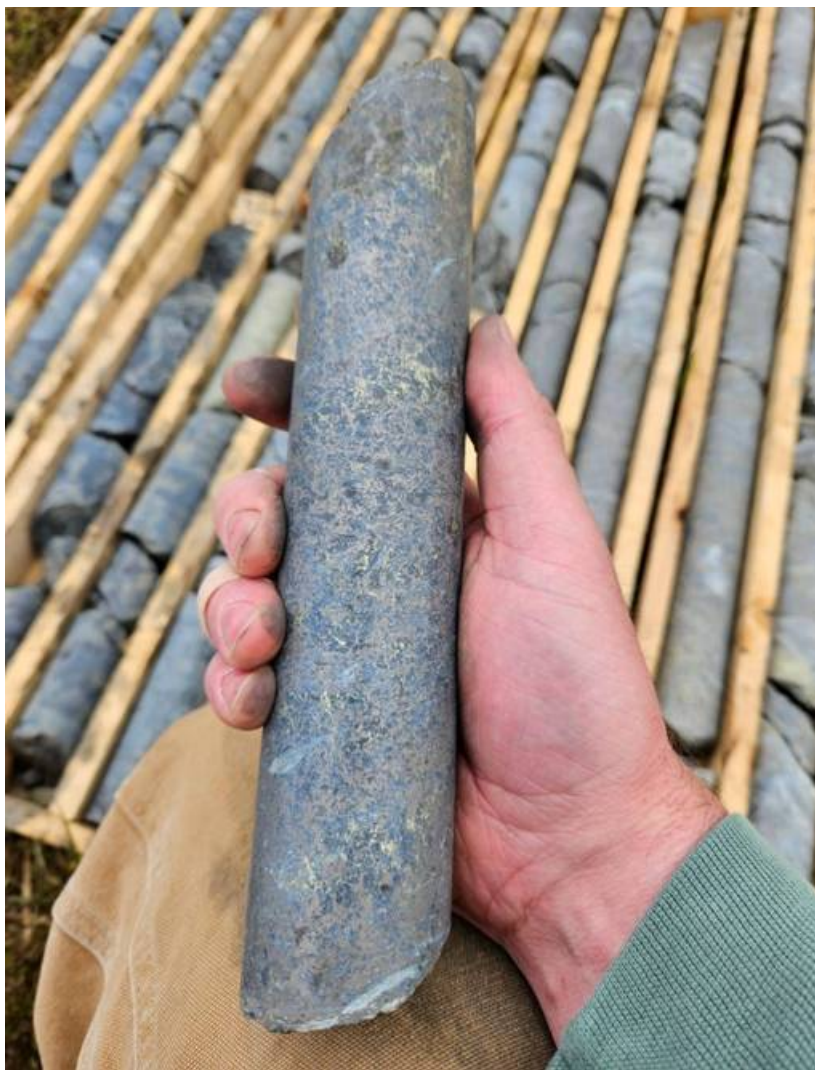
Figure 1: Part of a split section of drill core from hole 23-GL-01 showing massive sulphide.
