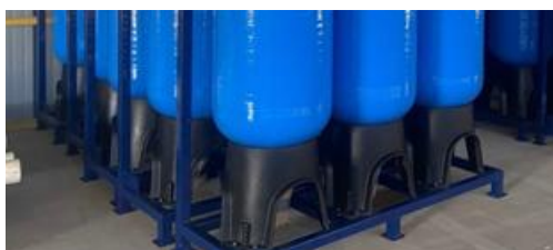
Fig. 7: Pilot plant DLE columns installed Copiapó (Aug 2023) Fig. 8: Rotary valve final tests Belgium (Aug 2023)
