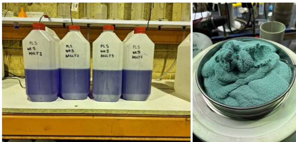
Photo 1: Week 3 - Pregnant Liquor Solution ("PLS") containers and copper-loaded Ion Exchange Resin
