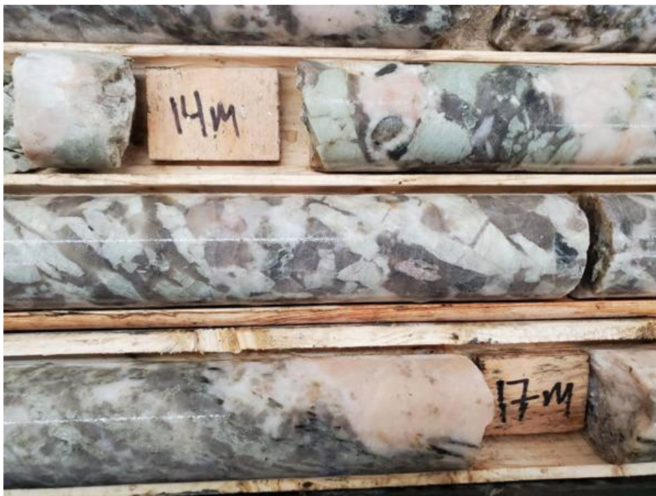
Photo 2 -Shallow intersection of pegmatite hosting spodumene (pale green 'blades' in hole ZIG-23-01).
