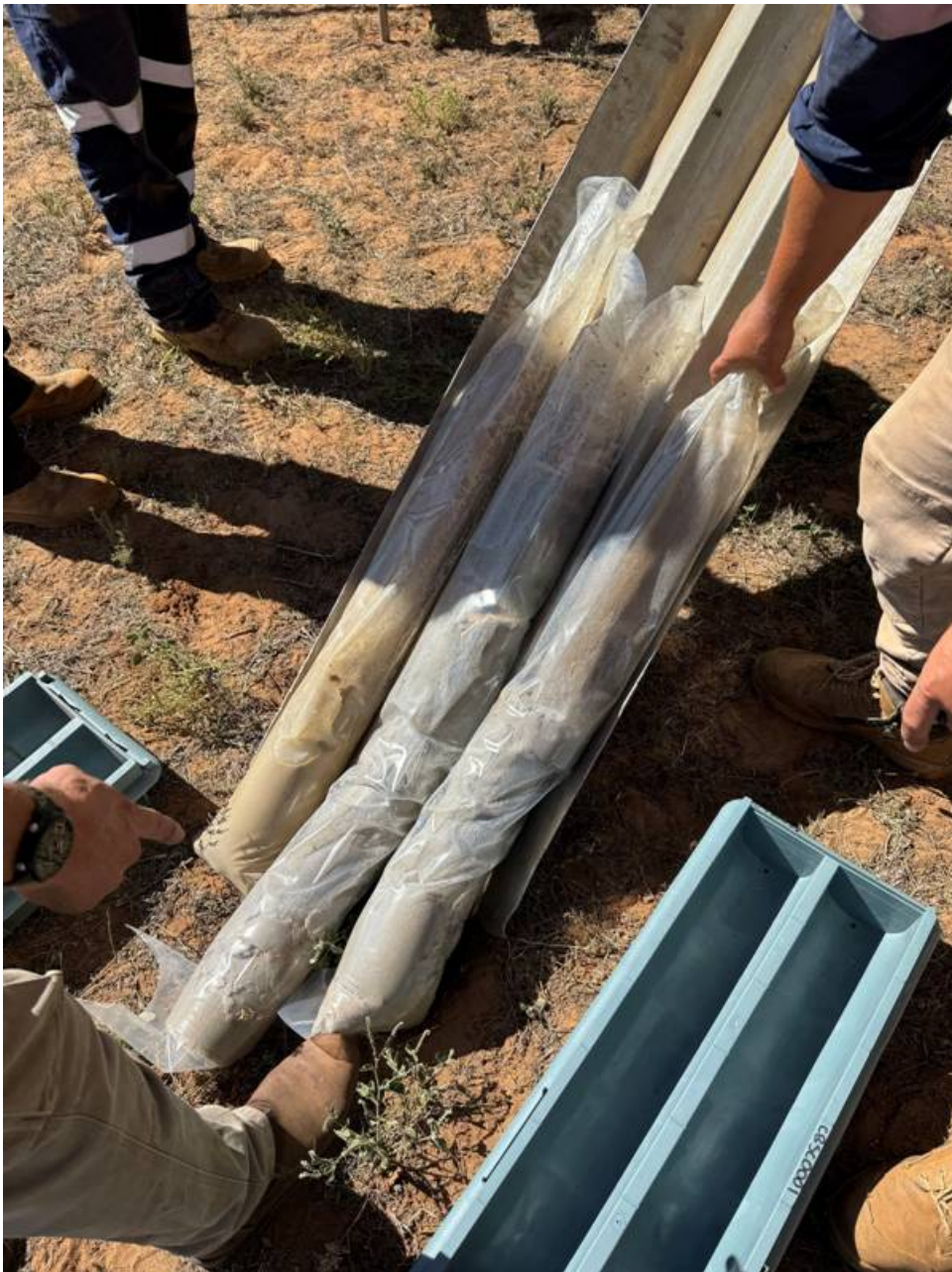
Figure 2: Core being recovered from sonic drilling at the Boland prospect
