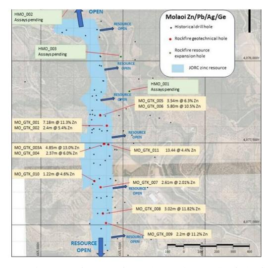
Plan view of the zinc resource (light blue colour), showing the location of historical drillholes (black dots), Rockfire geotechnical holes (red dots) and Rockfire resource expansion holes (green dots).
