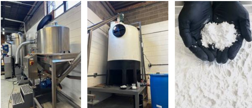
Figure 2: Conductive Energy - Milling and Refining Equipment, Continuously Stirred Tank Reactor, and Lithium Carbonate product in Chicago, USA (pictures left to right)
