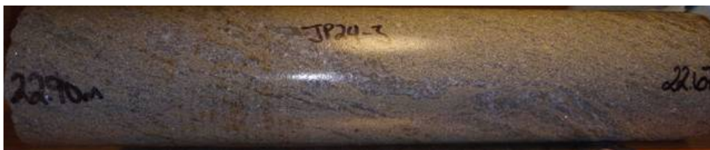
Figure 4: Core segment from recent drilling displaying massive pyrite parallel to foliation planes.
