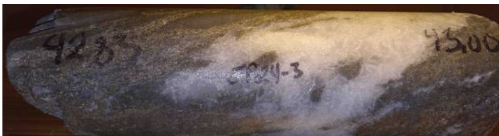
Figure 5: Core segment from recent drilling displaying a white quartz barite vein with sulphides along its margins.
