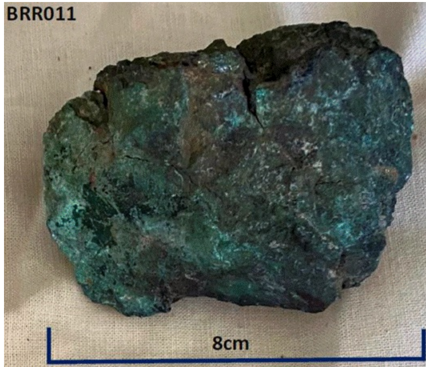
Figure 3: Rock sample BRR011 assayed at 49.9% Copper and 4.93g/t Silver (TechGen, 13 October 2021)
