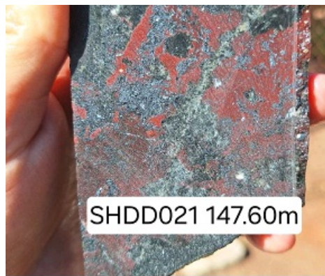
SHDD021 - Semi-massive hematite-magnetite iron mineralisation
