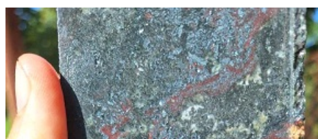
SHDD016 - Chalcopyrite-Pyrrhotite Mineralisation about 350m depth
