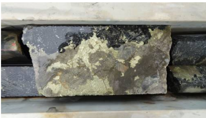
SHDD016 - Chalcopyrite-Pyrrhotite Mineralisation about 350m depth
