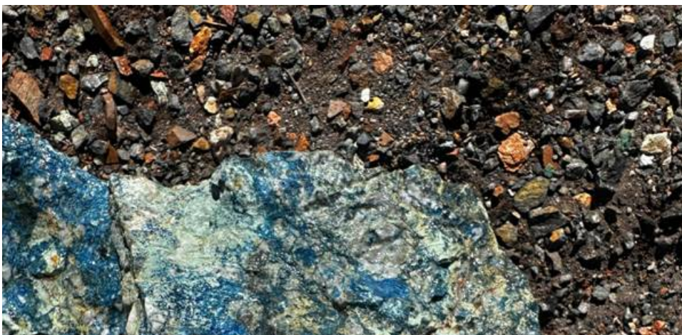
Figure 1: Photo of Rich Copper Oxide Sample from Historical Run of Mine pile next to Historical Shaft at Blue Rock Valley.
