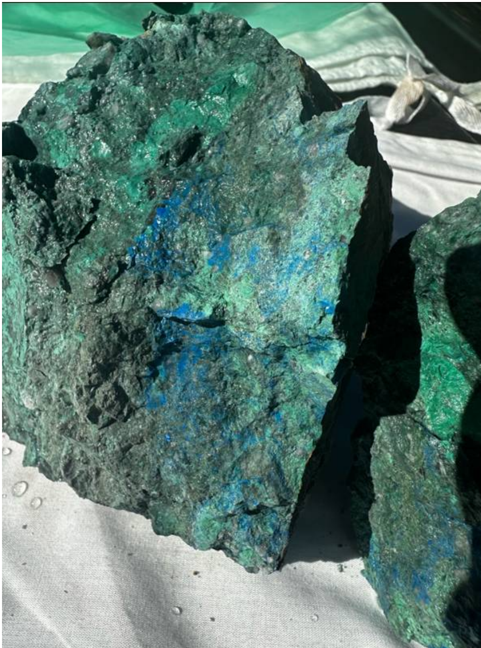
Figure 1: Photo of Rich Copper Oxide Sample from Historical Run of Mine pile next to Historical Shaft at Blue Rock Valley.
