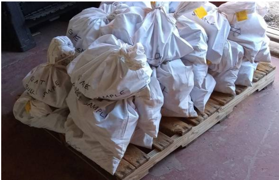
Figure 1: ~300kg bulk sample consisting of approximately 118m of half-core samples prepared for shipment to SGS Laboratory for advanced metallurgical testing.
