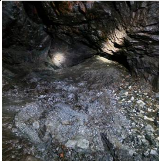
Figure 3: (left) part of new ladderway from No.4 Level down to No.5 Level; (right) some of the blasted material on 4.5 Level left behind from previous periods of mining (includes quartz vein right of photo)
