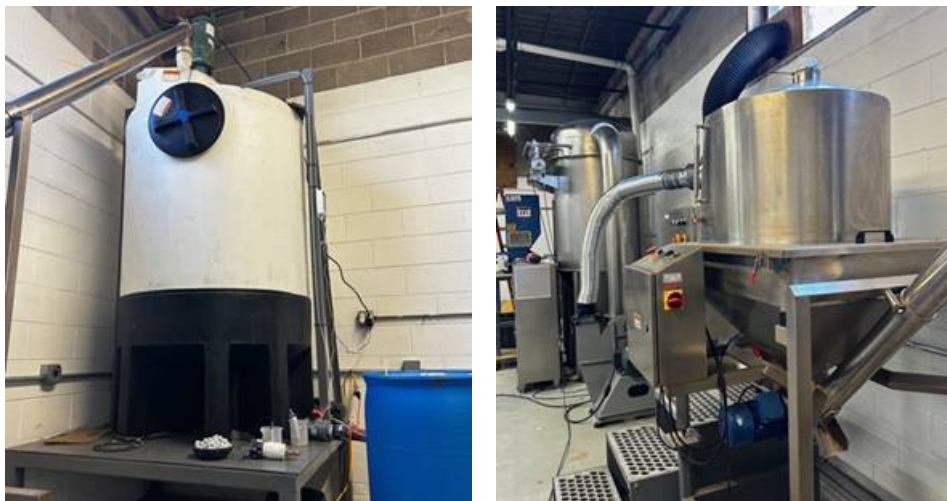
Figure 4: Conductive Energy Carbonation Reactor Tank and Equipment for Washing, Filtering & Drying
