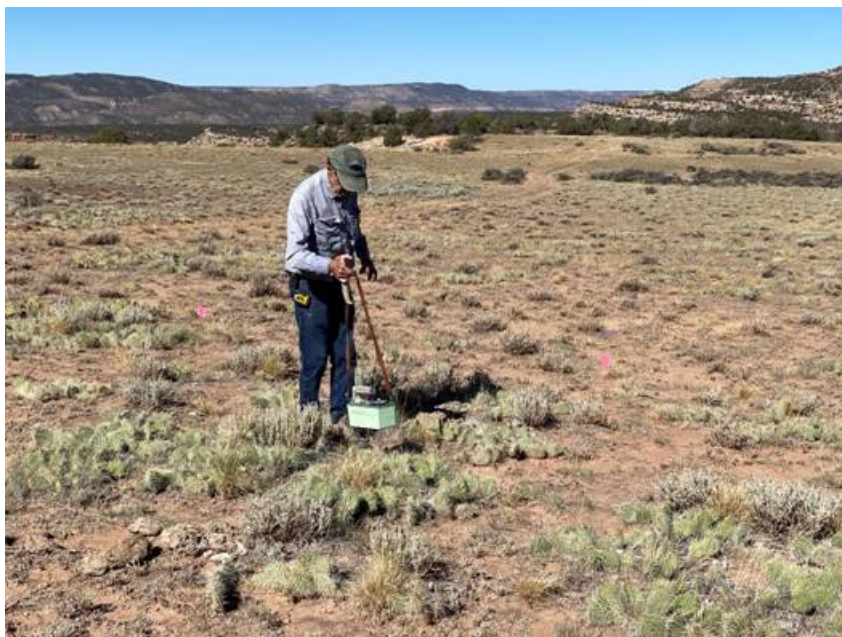
Photo 1: Collecting background Scintometer readings over proposed drill pads
