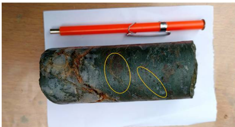
Figure 1: Drill core at the Kalayi Prospect (88.4m) showing strong chlorite alteration (green) and coarse grained cassiterite (red-brown mineral inside the orange ellipses).
