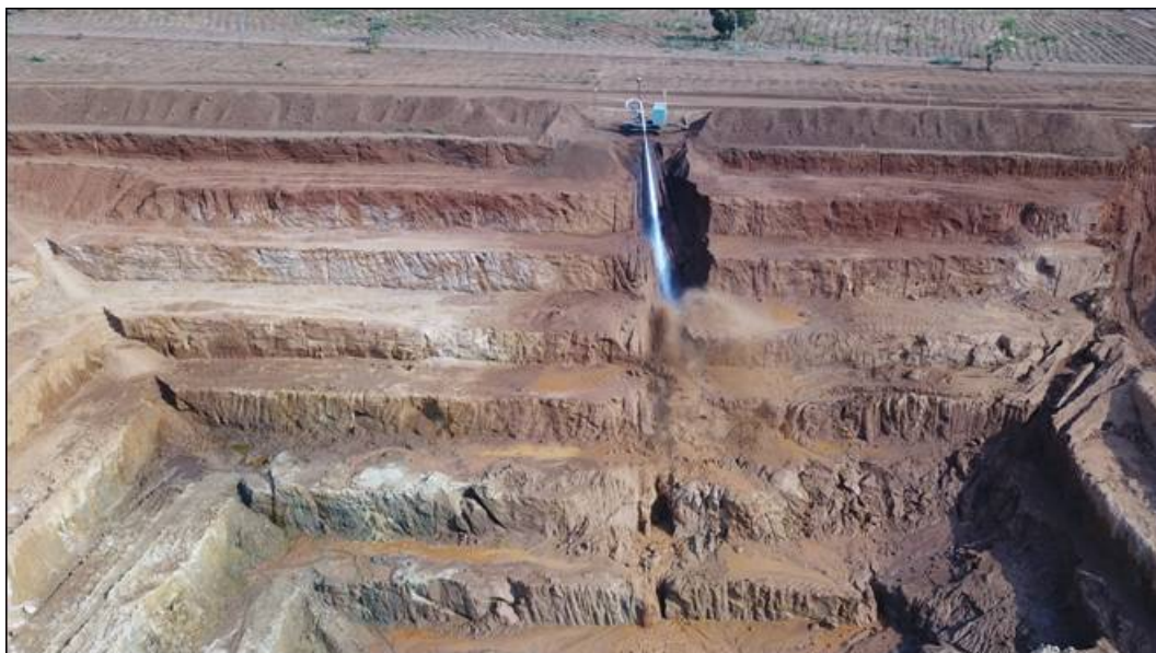
Figure 1: Hydraulic mined material (slurry) flows freely to the collection point in the bottom of the sump.
