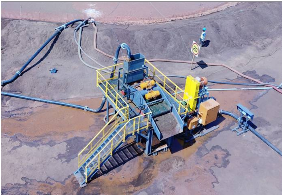
Figure 5: +2mm oversize is screened out using a vibrating screen.
