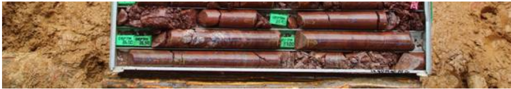
Figure 1: Drill core at the Kalayi Prospect showing strong weathered chlorite alteration (dark brown) and quartz veining. Visible cassiterite (tin oxide) observed on vein contacts.
