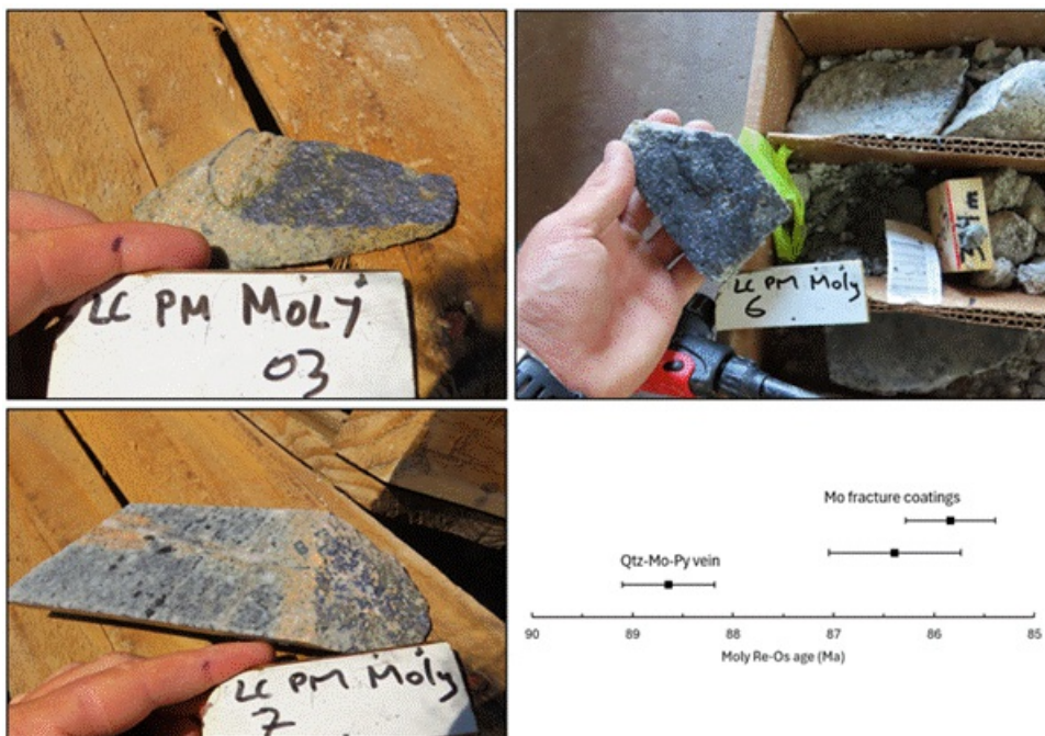
Figure 3: Photographs and Re-Os age determination of molybdenite samples collected from PM24-02.
