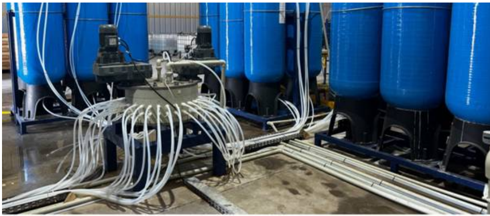
DLE Pilot Plant at R&D Centre in Copiapó, Chile (30 x approx. 3m columns to produce up to 1 tonne per month of LCE)
