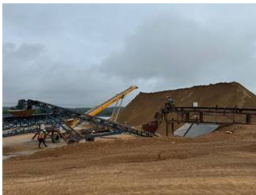
Stacking of agglomerated ore continues on Cell 5
