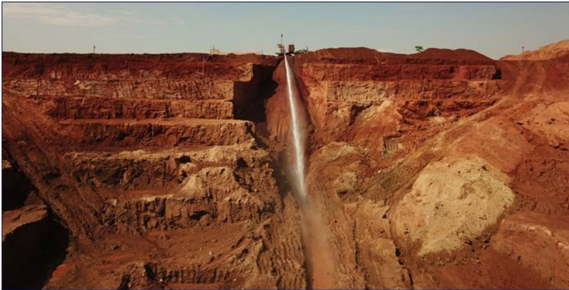
Figure 1: Hydraulic mining of Kasiya test pit
