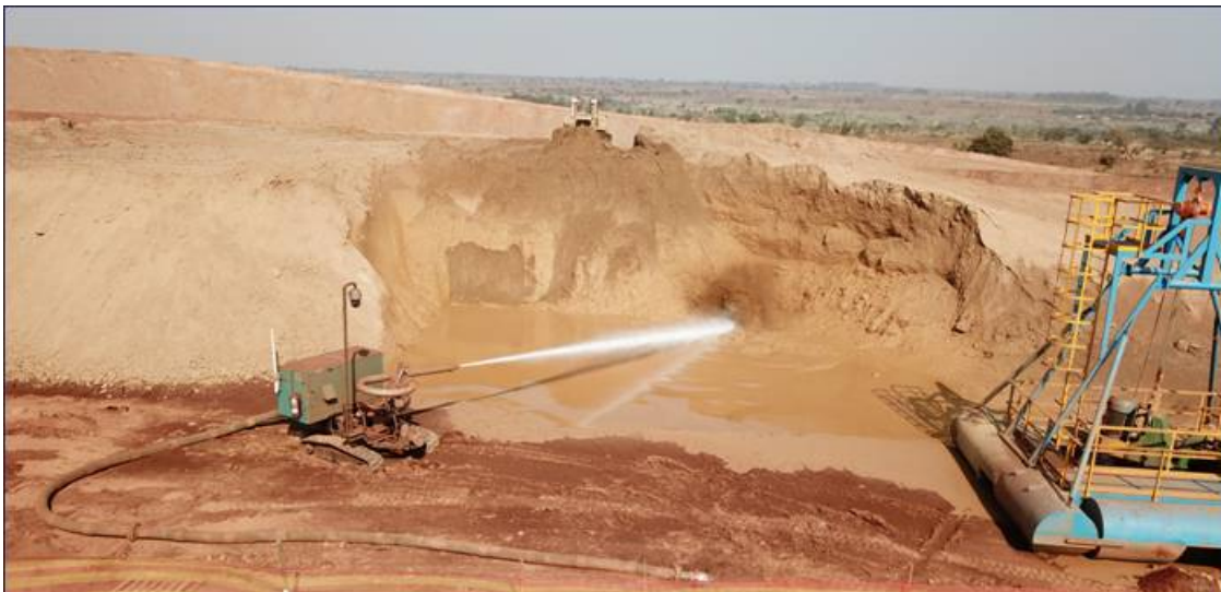
Figure 2: Water monitor demonstrating hydraulic mining of Kasiya material
