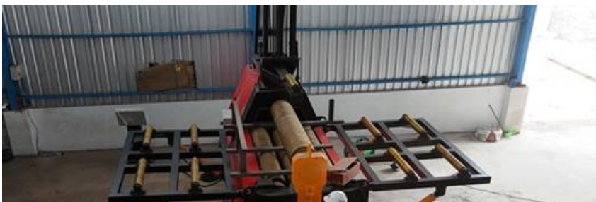
Photo 5: Inspecting 2m wide 4 roller press for rolling large plate steel for conveyor pulleys and tank sections.
