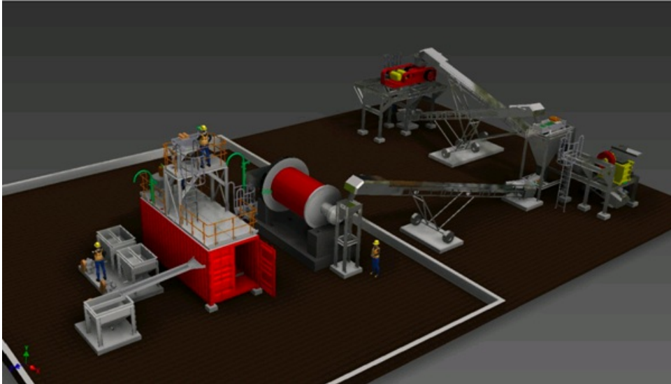
Figure 4: Illustrative layout of 100t/d CIP gold processing plant
