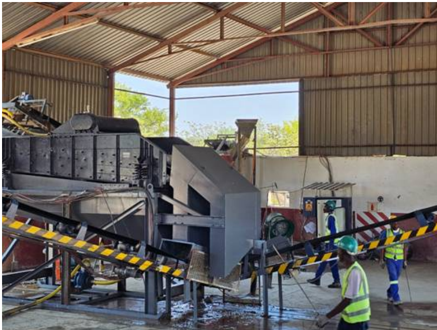
Figure 1. New Double Deck vibrating washing and sizing screen in operation
