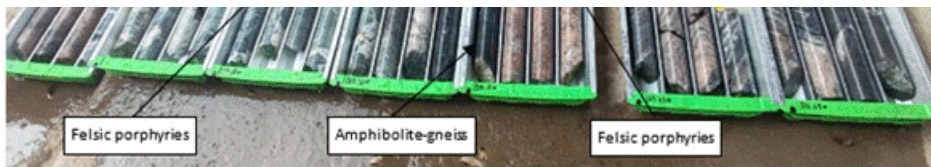
Figure 2. Example of drill core from MBD001 showing the amphibolite-gneiss host rock, intruded by felsic porphyries (quartz-feldspar porphyries). Areas of K-feldspar alteration are apparent within individual QFP intrusions.
