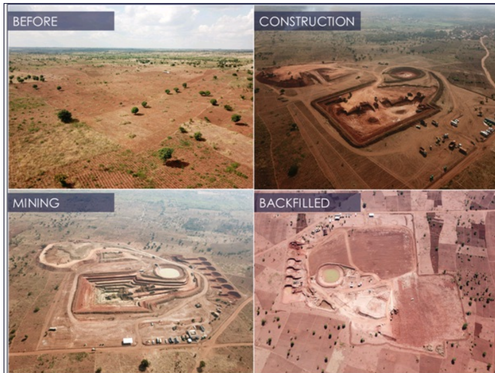
Figures 2-5: Stages of test pit mining and backfilling
