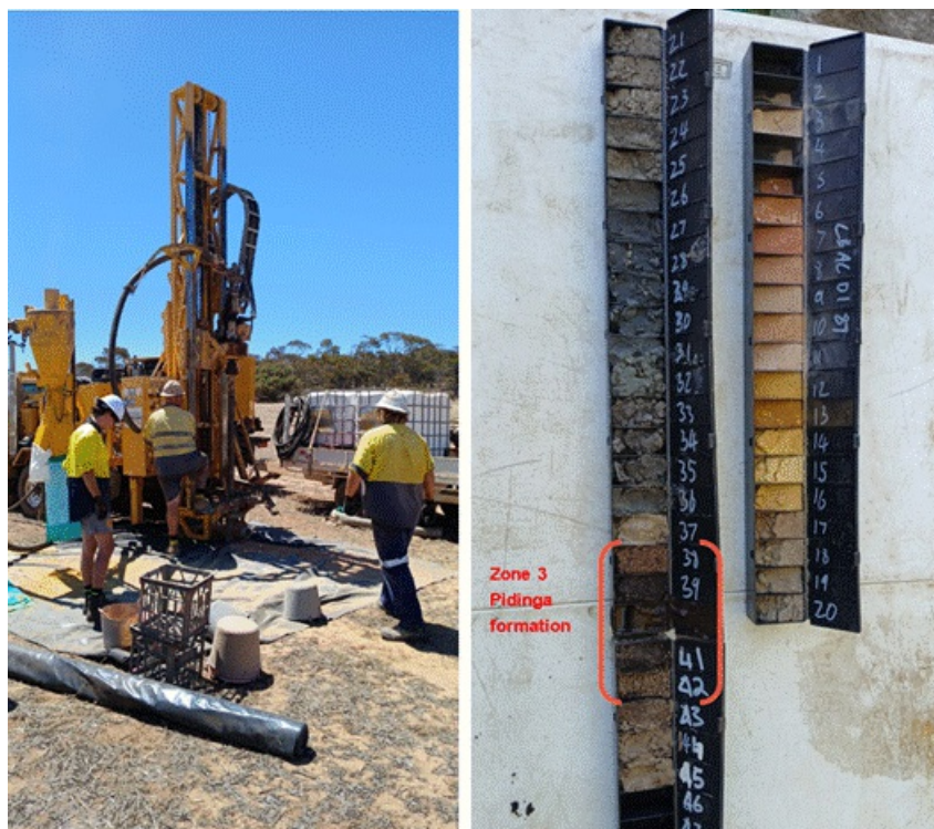
Figure 1: (A) Aircore drilling underway at the Boland Project. (B) Aircore chips from drillhole CBAC0187 defining the geological target (Zone 3) - reduced organic rich Pidinga Formation containing coarse, permeable sands 38 - 42m
