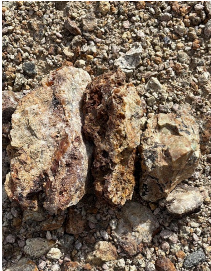
Figure 1: Sample CJ0079 showing classic quartz-colloform low-sulphidation epithermal textures.
