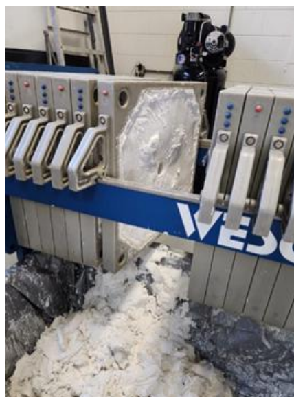
Image 4: Filter press used in the conversion process to produce lithium carbonate
