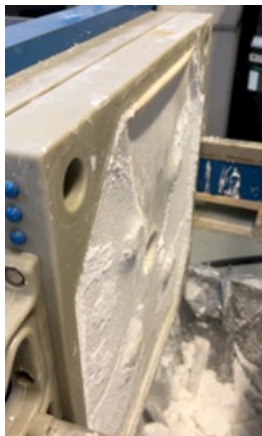
Images 1-2: High purity lithium carbonate falling from filter plate and final product. Low adhesion and moisture content is an indicator of high product purity & exceptional crystal structure
