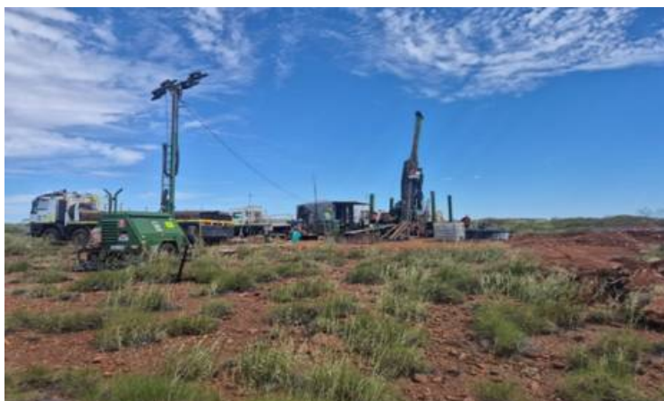
Figure 1. Diamond drill rig set up on the first hole at Carlow. Drilling 24hrs/day
