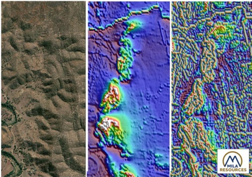
*Figure 1: Snapshot of geophysical data gathered during the recent ground magnetics survey. The data provides a large advance on the last survey, which was completed in the mid-90s and allows modern processing techniques to define key controls and features associated with gold mineralisation.*
