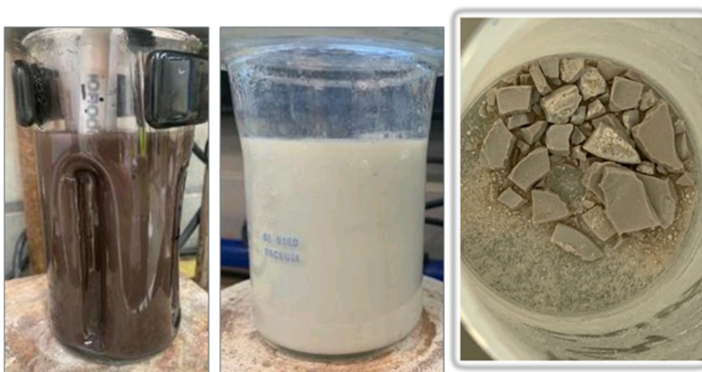
Figure 2. Purification and product finishing testwork, photos from left to right: titanyl sulphate solution from leaching stage, hydrated TiO 2 produced from hydrolysis, and the calcined TiO 2 product.
