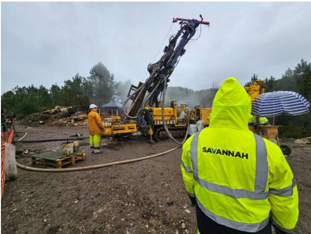
Figure 2. Recent Reverse Circulation drilling at Pinheiro
