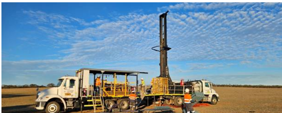
Figure 1: Sonic drilling underway at the Boland Project
