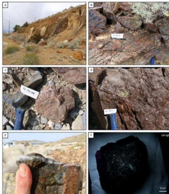
Figure 2: (A) looking north at outcropping circa 20 m thick skarn zone at the contact between intensely QSP altered quartz monzonite (right) and limestone (far left). This outcrop is above a glory hole into an open stope, the same seen in Figure 1 D. (B) example of outcropping banded garnet (red) and pyroxene (green) skarn. (C) sample of coarse garnet skarn, with garnets up to 1 cm in diameter. (D) pods of massive sulphide in garnet skarn. (E) banded skarn cut by chalcopyrite-pyrite mineralised quartz vein. (F) fluorescence under UV light of garnet skarn showing high concentration of powellite and/or scheelite. Gn = garnet, Py = pyrite, Cpy – chalcopyrite, Qtz = quartz, Px = pyroxene.
