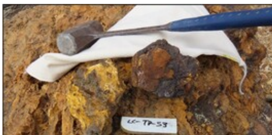
Figure 6: Examples of outcropping molybdenite-pyrite-quartz veins in the QSP altered southern quartz monzonite stock, demonstrating hypogene porphyry-style mineralisation. Mo = molybdenite, Py = pyrite, Qtz = quartz.
