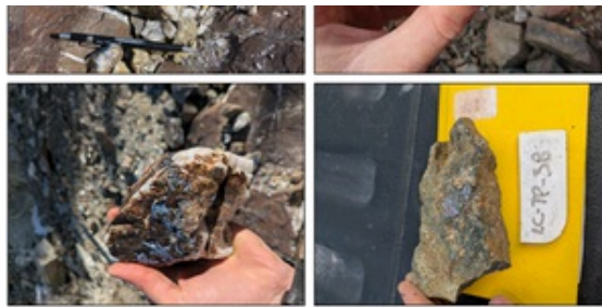
Figure 3: Examples of coarse grained molybdenite mineralisation in garnet skarn, found associated with calcite veins at and near the contact between the skarn with unmineralised hornfels.
