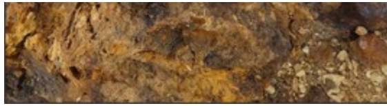
Figure 7: Sample of gossanous, massive sulphide mineralisation adjacent to outcropping stockwork quartz-sulphide veins in QSP altered quartz monzonite.
