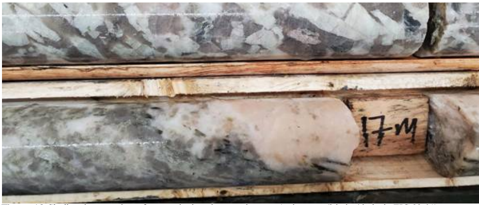
Figure 18 -Shallow intersection of pegmatite hosting spodumene (pale green 'blades' in hole ZIG-23-01). Two (shallow) step-back holes were conducted as well as a scissor hole to confirm the dip of the structure. Further drilling is warranted both along the (open) strike to the west and east as well as down dip.
