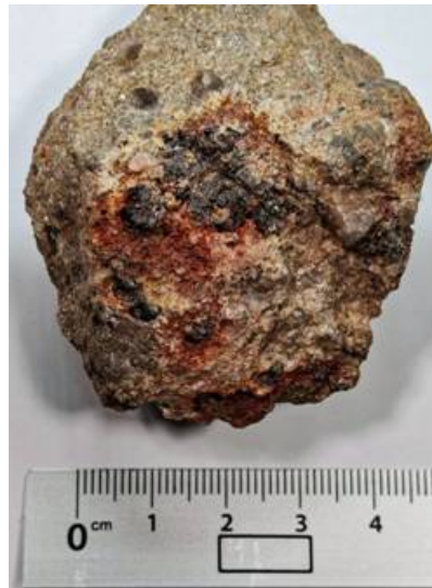
Figure 6: Rock chip sample showing coarse cassiterite (black mineral, \text{SnO}_2 ) from St Michaelis structure
