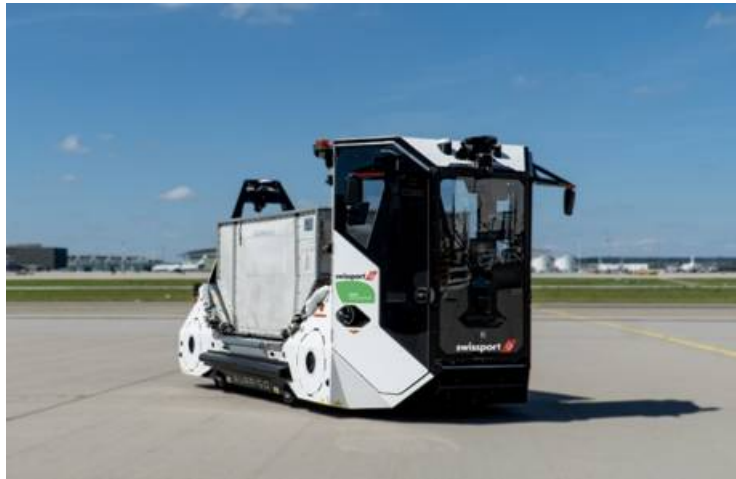
Image: Auto-DollyTug®, a fully autonomous baggage and cargo handling vehicle
